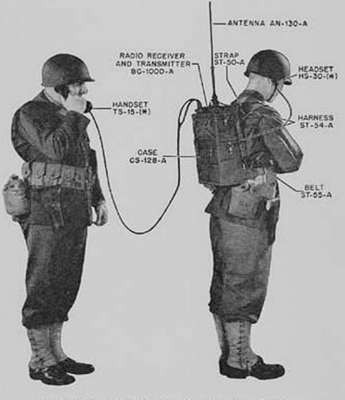
Figure 1. Radio Set SCR-300-A. In Use, Viewed From Right Side,
